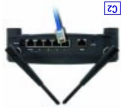
If you are connecting more than four PCs to the Router, you will need to connect a hub or switch to the Router's Uplink port (if you use the Router's Uplink port, then you cannot use Port 1). For information on Uplinking, please refer to the User Guide located on the Setup Wizard CD-ROM.
