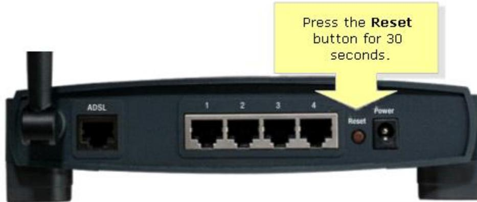
**Figure 2:** Location of the **Reset** button of a Linksys WAG54G v1 ADSL gateway.
