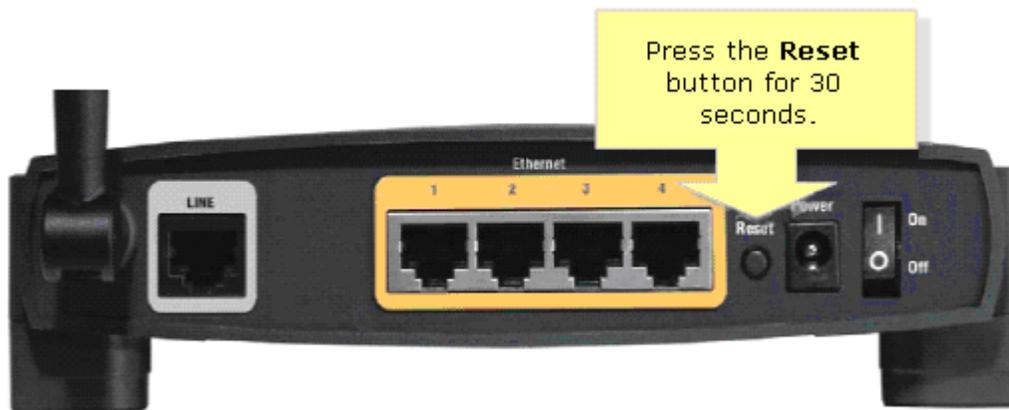
**Figure 3:** Location of the **Reset** button of a Linksys WAG54G v1.2 ADSL gateway.
